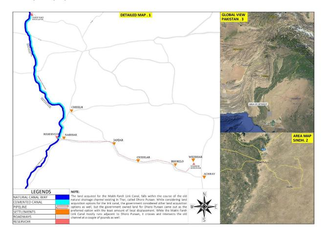
Makhi-Farsh Link Canal is a freshwater supply scheme being implemented by the government of Sindh which proposes to provide 200 cusecs of freshwater to Thar Coalfields via a 70-kilometer-long Concrete Channel (CC). This CC/Link Canal/Makhi Farash Link Canal starts from Farsh Mori, a water regulator, at Makhi Farsh Canal near Dhoronaro in district Umerkot and ends at Nabisar and from there it is further stretched to Vejhiar through 60-kilometer pipeline in district Tharparkar.
